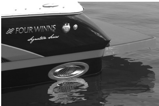
Figure M13: Thru-Hull Exhaust
