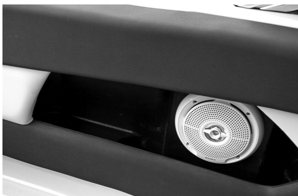
Figure N25: Port Coaming Pad with Sidewall Storage (Representative View - Models May Vary)
