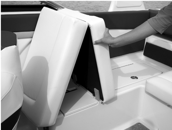
Figure M18: Hinged Seat Cushion - Certain models Only (Creates Step & Provides Access to Storage)
