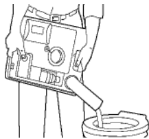
Figure J15: Emptying Waste Holding Tank
