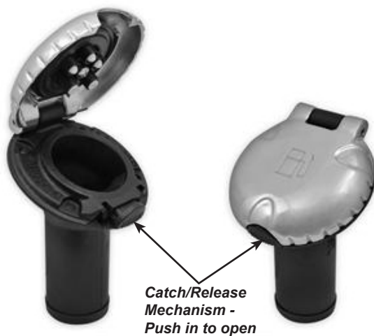
Figure 15: Fuel Deck Fill Catch/Release Mechanism
