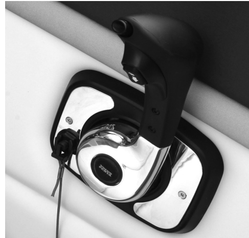
Figure A1: Throttle Control in Neutral Position
