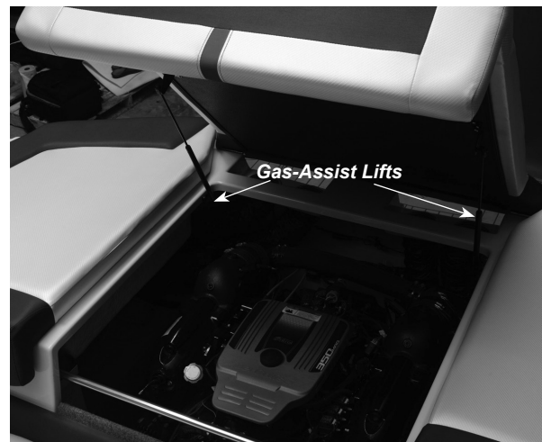
Figure N20: Raised Center Sundeck - Engine Compartment Access (Representative View - Models May Vary)
