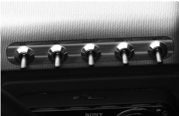
Figure H9: Helm Switch Panel - Starboard View
