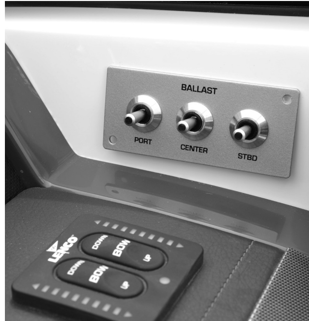
Figure L16: Ballast System Switch Panel
