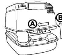
Figure J9 (A-B) : Removing Fresh Water Tank
