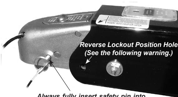
Always fully insert safety pin into coupler latch (hole) prior to towing.
