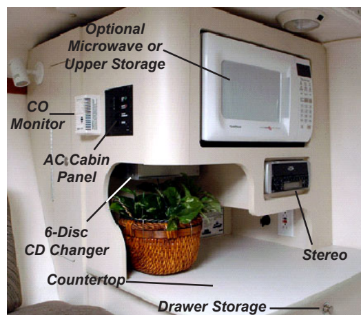
Figure H3: AC Cabin Panel Locations
