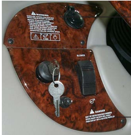
Imprinted Labels on Port Ignition Panel
