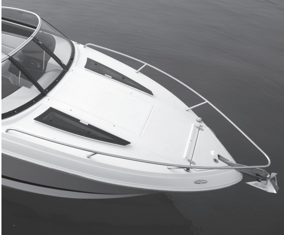
Figure M1: Deck Rail - Standard Height
