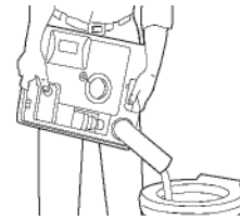
Figure J11: Emptying Waste Holding Tank
