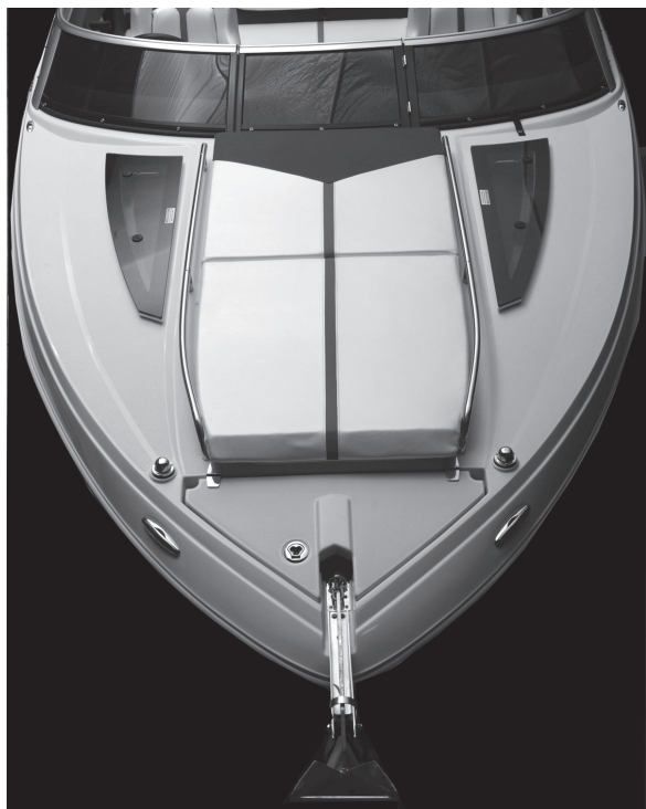
Figure M2: Deck Rail - Low Profile
