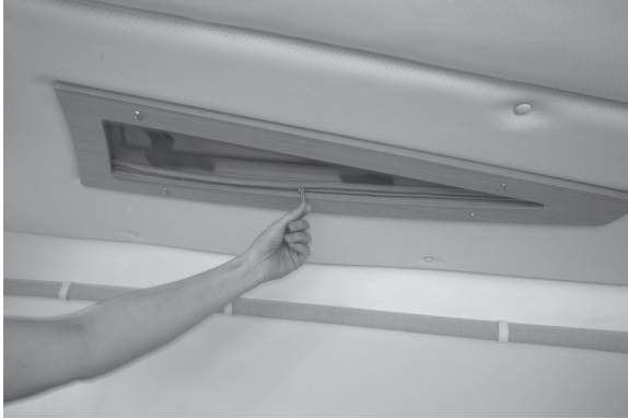
Figure Q4: Wood Trim - Deck Hatch
