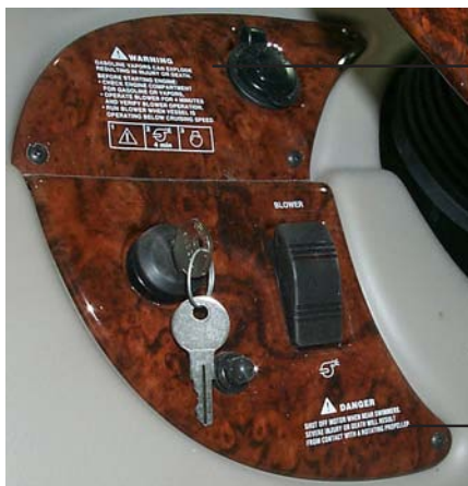
Imprinted Labels on Port Ignition Panel
