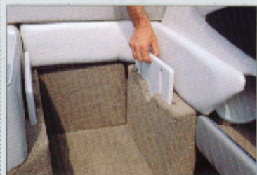
Jump seat supports lift & lock...
