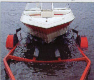
Convenient positioning of side guides, angled bunks, and a recessed frame-mounted roller make it easier to drive the boat onto the trailer.
