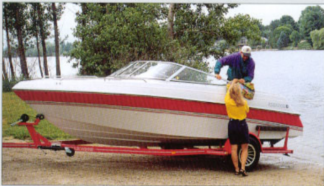
A low profile aids at launch time, often allowing the boat to be floated off the trailer.
