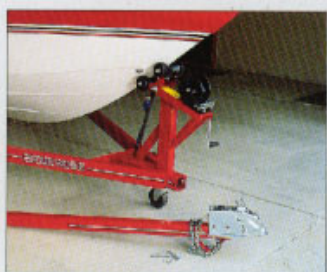
Removable tongue is handy for storage and as a security feature.
