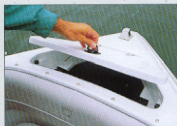
Anchor locker w/anchor cradle.
