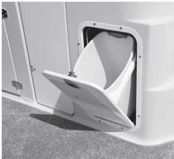
Figure J5: Trash Receptacle - Port Console
