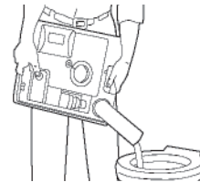
Figure J15: Emptying Waste Holding Tank
