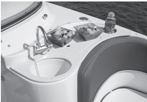
Figure L2: Integrated Sink, Cooler & Trash Receptacle
