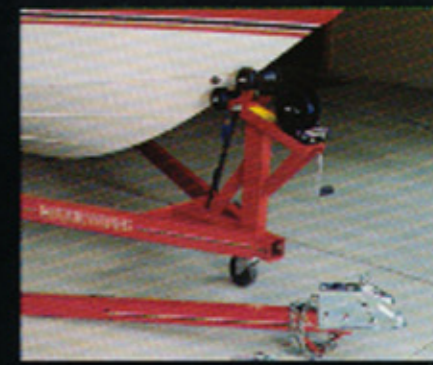
Above left - a zinc chromate primer and two coats of color-matched polyurethane paint give the trailer its long-lasting good looks.
