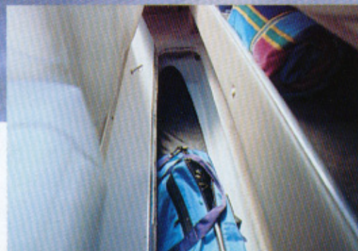
A ski locker integrated into the cockpit floor is part of the standard seating package.
