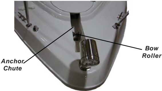
Figure M11: Anchor Chute and Bow Roller
