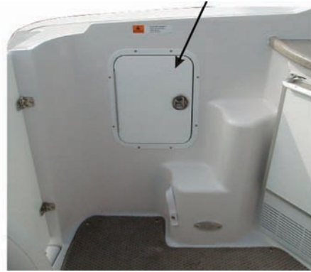
Ships System Door (Battery Switch & Breakers Inside)
