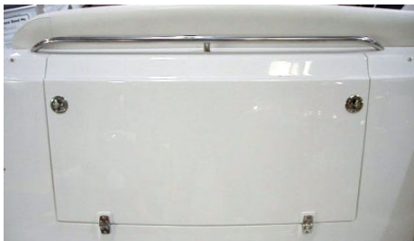
Figure M9: Transom Storage Locker
