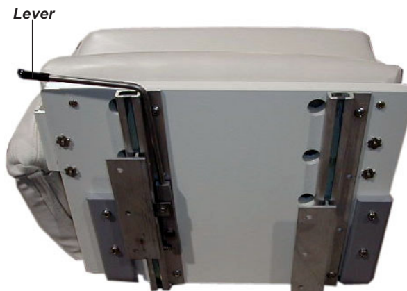
Figure N5: Helm Seat Slider Mechanism
