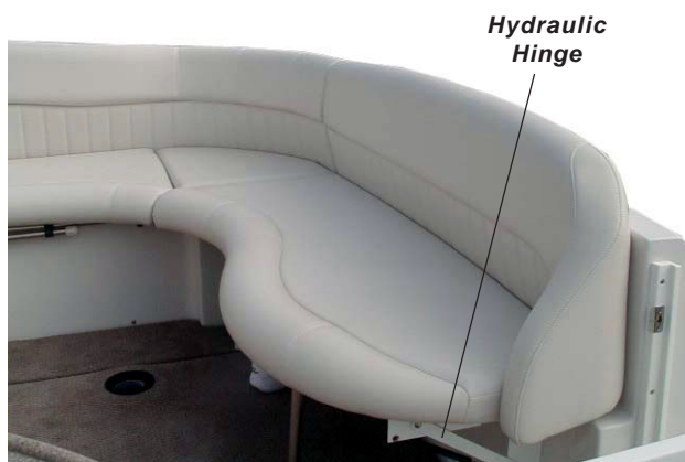
Figure N11: Aft Cockpit Stern Seat w/ Hinge Assembly
