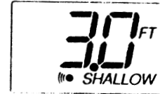
Figure E7: Shallow Alarm Setting Value
