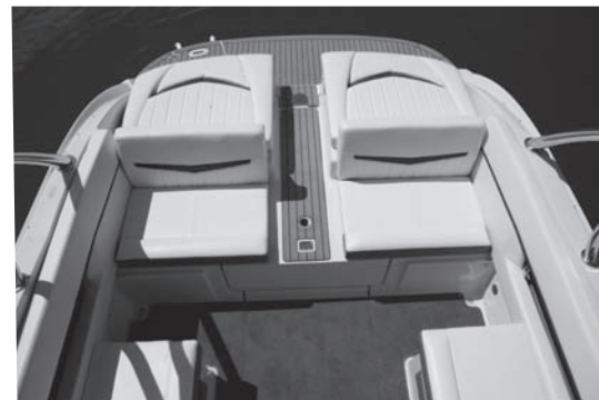
Figure N12: Jumpseats in Stored Position
