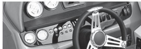
Figure Q4: Helm Switch Panel
