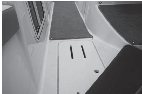
Figure L11: In-Floor Storage Locker
