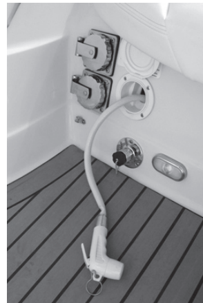
Figure J3: Aft (Transom) Shower
