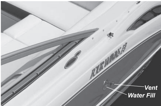
Figure J1: Water Fill
