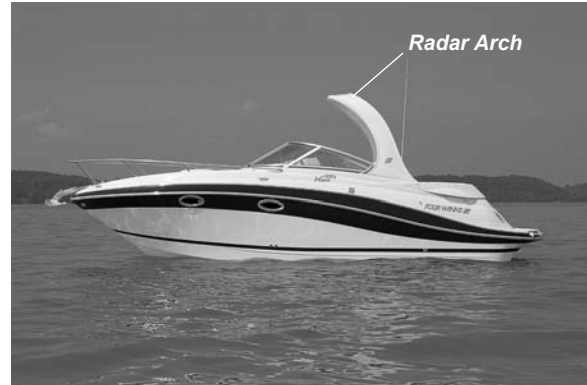
Figure M14: Radar Arch
