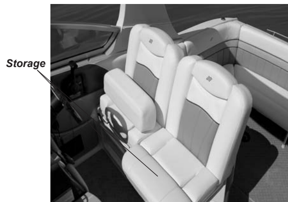
Figure M9: Cockpit Storage Compartments (Note: Bolsters flip-up for access to storage compartments).
