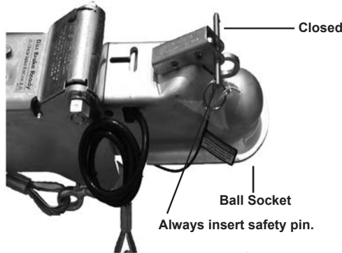
Figure S7: Surge Brake Actuator & Coupling Assembly
