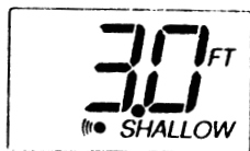
Figure E9: Shallow Alarm Setting Value
