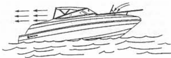
FIGURE H5: DESIRED AIR FLOW THROUGH THE BOAT.
