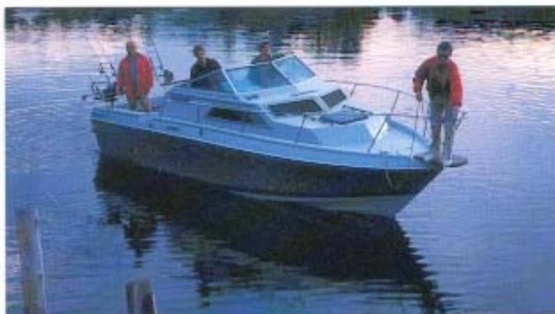
Standard bow pulpit reached by non-slip deck and welded stainless steel rails.
