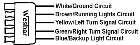
Figure R7: 5-Wire Plug Harness
