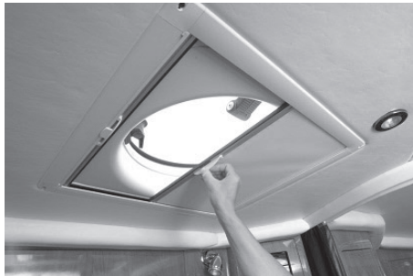
Figure K1: Layered Deck Hatch Screen/Sun/Shade System
