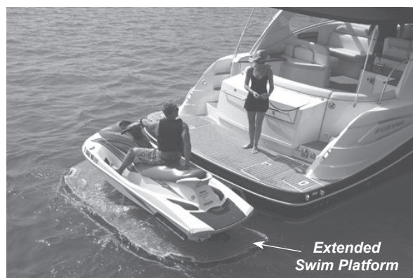
Figure M16: Extended Swim Platform Lift (Certain Models Only)
