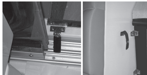
Figure M4: Companionway Door Keepers
