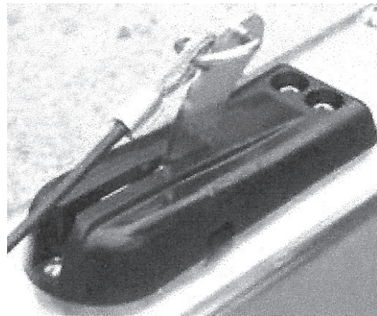
Figure S16: Emergency Break-Away Normal Position
