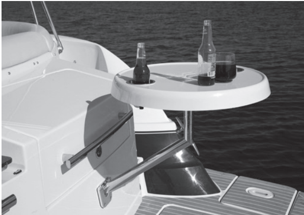
Figure M23: Transom Table Installed
