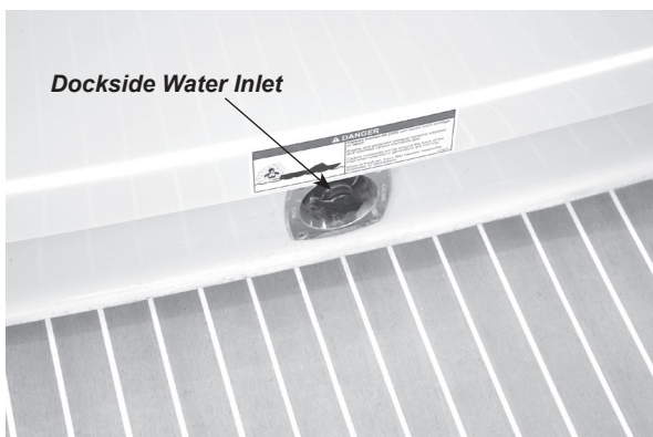
Figure J8: Dockside Water Inlet
