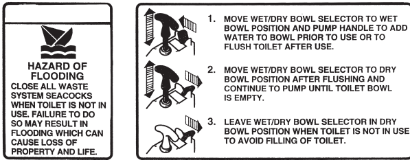
Figure J12: Wet/Dry Toilet Operations Label
