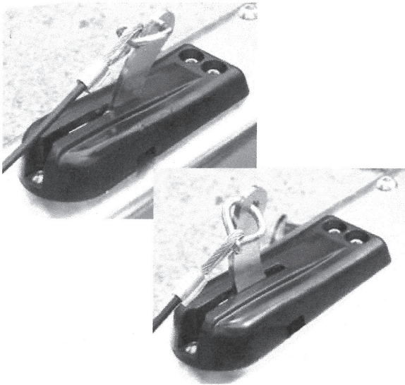
Figure S13: Emergency Break-Away Normal & Engaged
