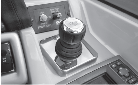
Figure F7: MerCruiser's "Axis" Joystick
