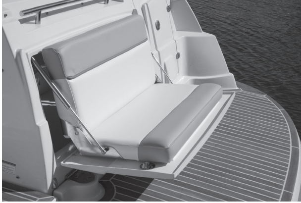
Figure N30: Swim Platform Seat - N/A All Models (Stores in Transom Storage Compartment when not in use.)
