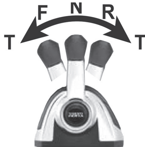
Figure A6: Control Lever Positions - Dual Binnacle (Representative View - Models may vary)
