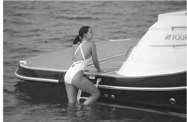
Figure M9: Starboard Boarding Ladder Shown (Typical Port & Starboard)
