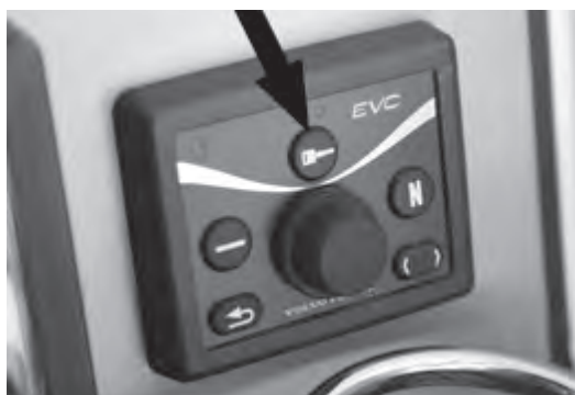
Figure A4: EVC Control Panel Activation Button
