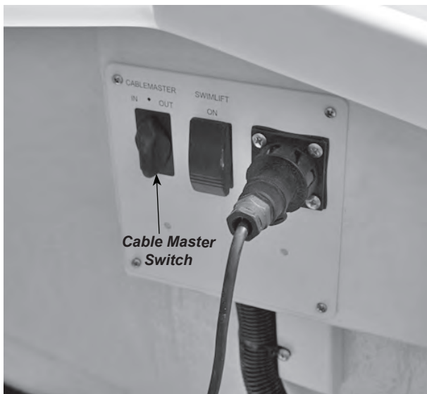
Figure H19: Cablemaster Switch Location
