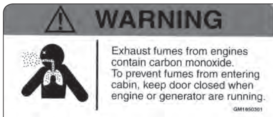
Carbon Monoxide - Cabin Doors Warning Label
