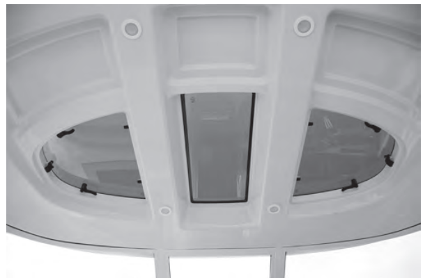
Figure K7 Hardtop w/Skylights
