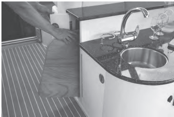
Figure N21: Aft Cockpit Table Storage
