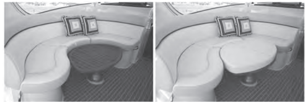
Figure N23: Port Lounge Converted to Berth
