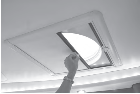
Figure M7: Screen/Shade System
