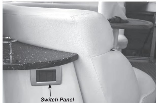
Figure N24: Task Lights & Table Switch Panel
