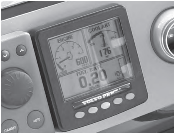
Figure E10: EVC System Display
