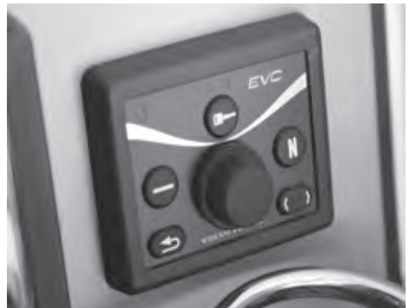
Figure E11: EVC Control Panel
