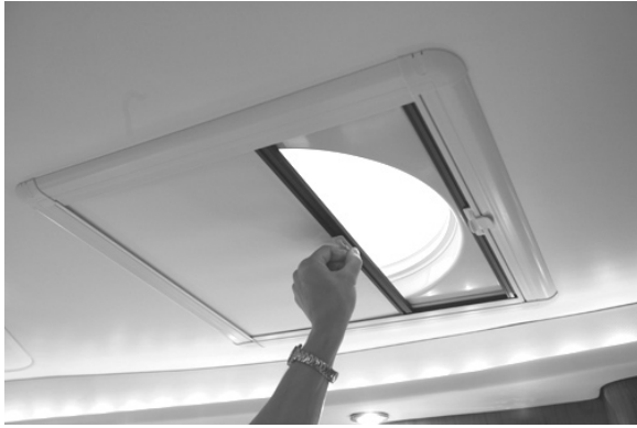
Figure M7: Screen/Shade System
