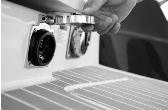
Figure L17: Phone/Cable TV Dockside Inlet Location
