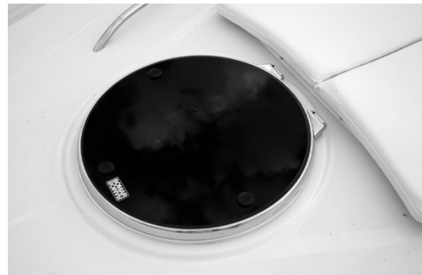
Figure K1: Deck Hatch
