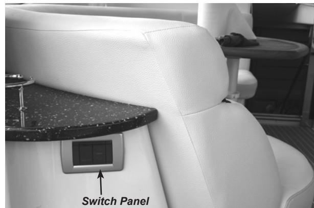
Figure N24: Task Lights & Table Switch Panel
