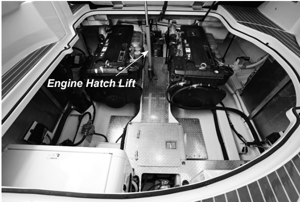
Figure M22: Electric Lift for Engine Hatch
