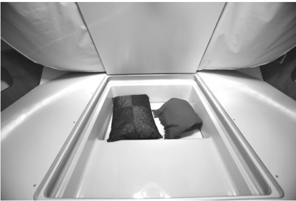
Figure N7: Under Berth Storage
