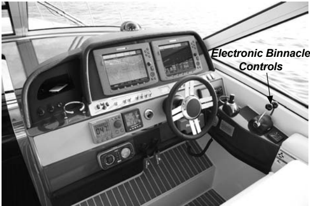
Figure F1: Helm Station
