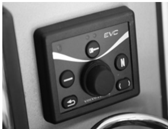
Figure E11: EVC Control Panel
