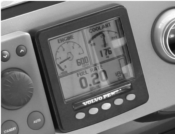
Figure E10: EVC System Display
