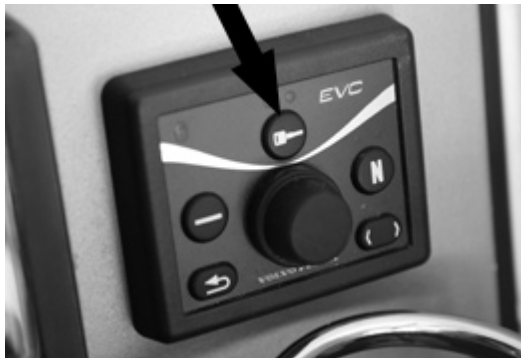
Figure A4: EVC Control Panel Activation Button
