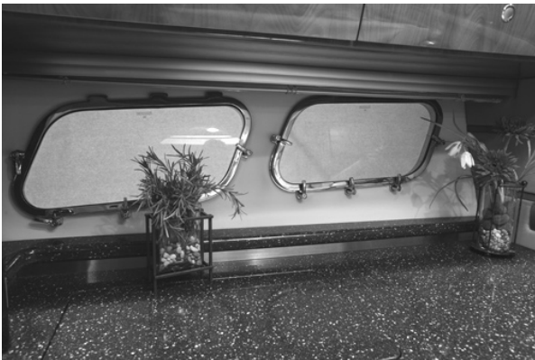
Figure K4: Side (Portlight) Windows at Galley
