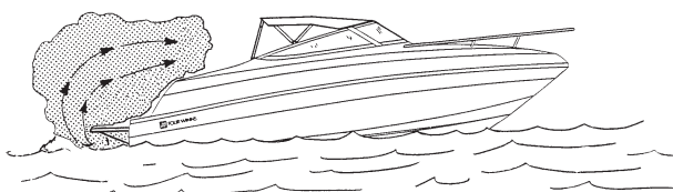
Figure B13: Exhaust Gas Accumulation at Swim Platform
