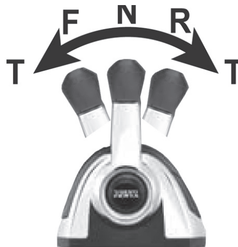
Figure A6: Control Lever Positions - Dual Binnacle (Representative View - Models may vary)
