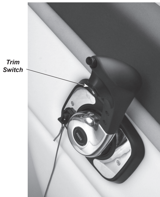
Figure F1: Side-Mount Control - Single Engine (Representative Image only - Models may differ)
