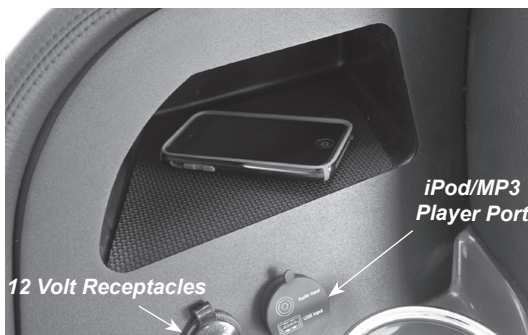
Figure H19: 12 Volt Receptacles & iPod/MP3 Player Port (Representative View - Models May Vary)
