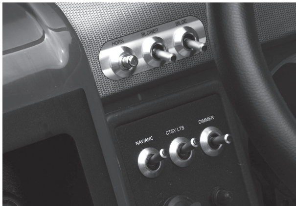
Figure H8: Helm Switch Panel - Port View
