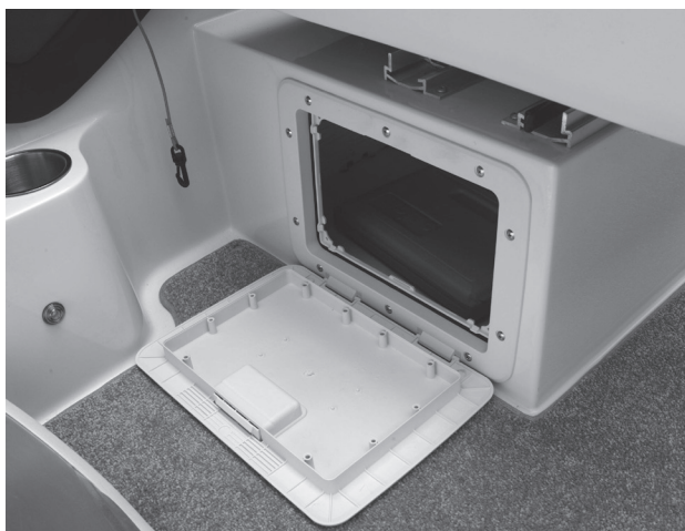
Figure L13: Storage Compartment Under Helm & Passenger Seats - Helm Storage compartment shown.
