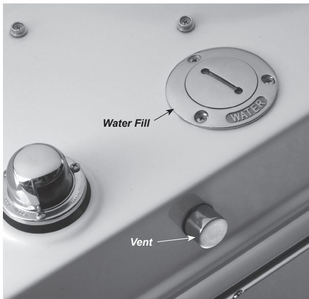
Figure J1: Water Fill & Vent
