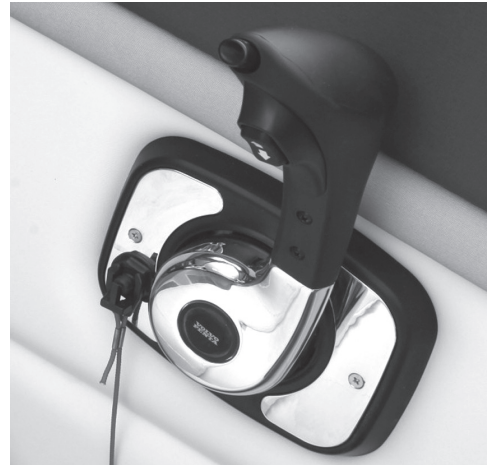
Figure A1: Throttle Control in Neutral Position
