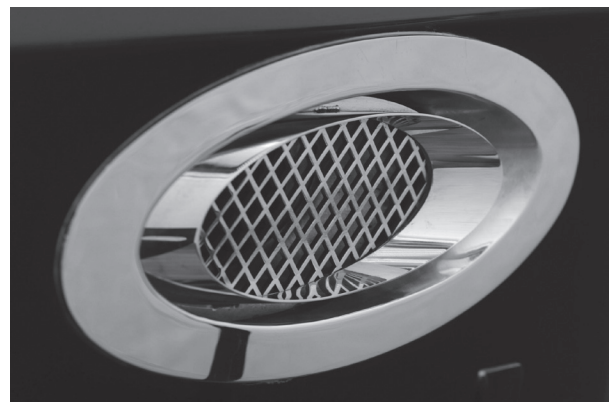
Figure M13: Thru-Hull Exhaust
