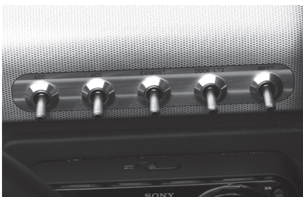
Figure H9: Helm Switch Panel - Starboard View
