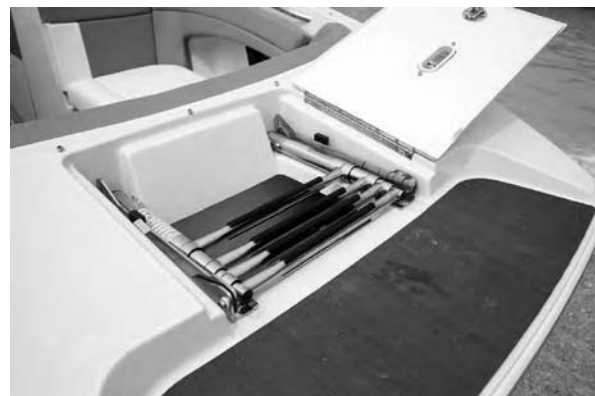
Figure L8: Anchor Locker w/Hidden Ladder
