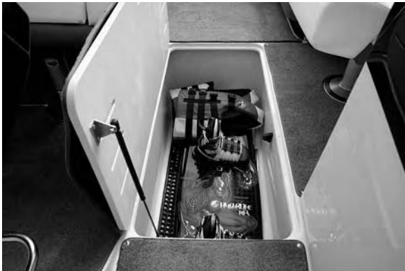
Figure L10: In-Floor Storage Locker
