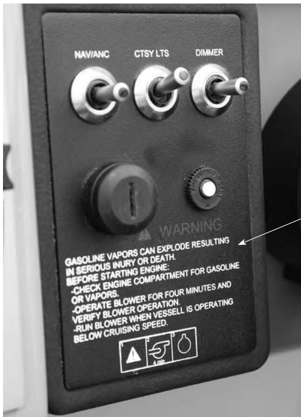
Imprinted Label on Ignition Panel
