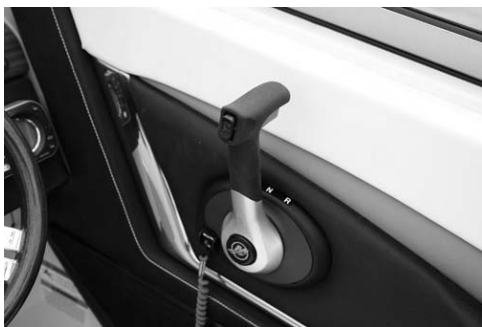
Figure A1: Throttle Control in Neutral Position
