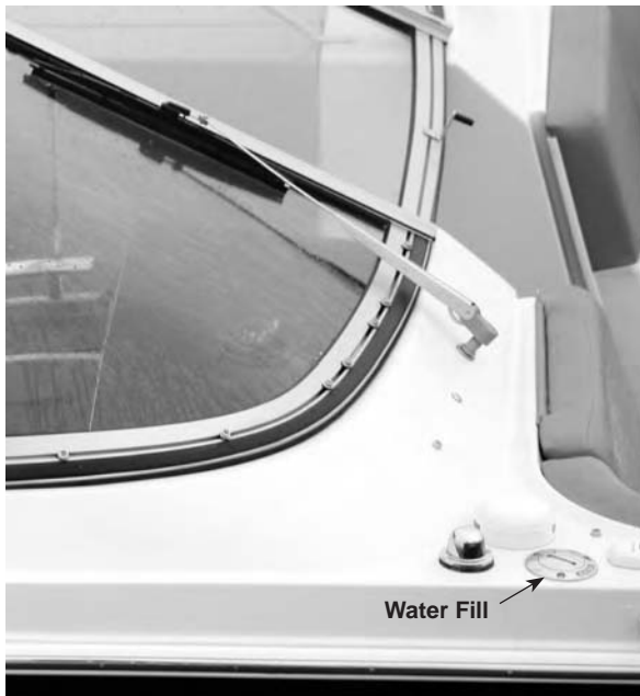
Figure J1: Water Fill
