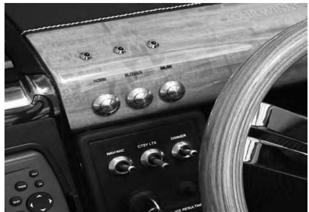
Figure H6: Helm Switch Panel - Port View
