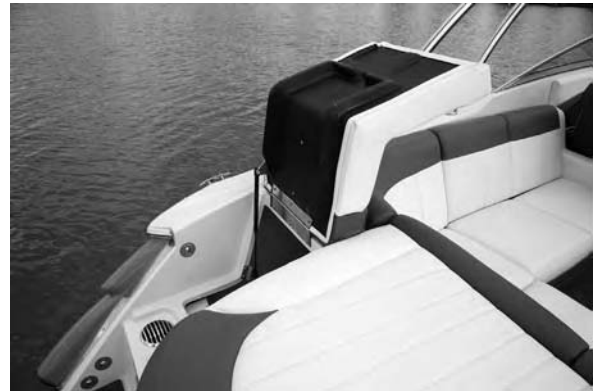
Figure L11: Port Aft Deck Storage Locker To Access: Lift Up on the Port Transom Seat (if applicable). (Note: Certain Models Only - Models May Vary)
