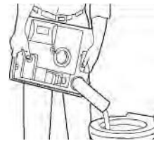
Figure J11: Emptying Waste Holding Tank
