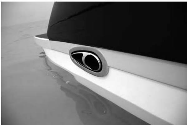
Figure M10: Thru-Hull Exhaust
