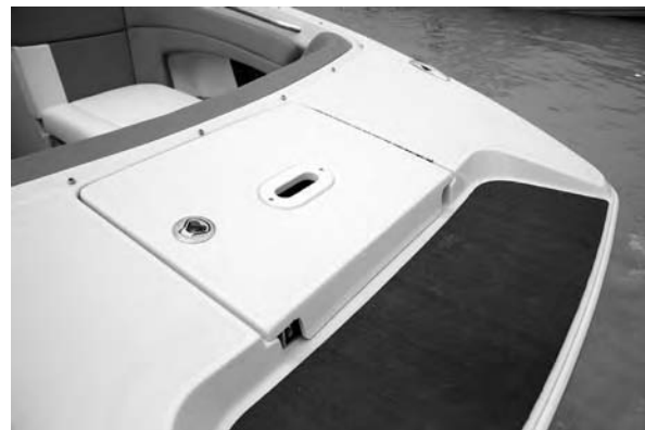
Figure M8: Integrated Bow Platform
