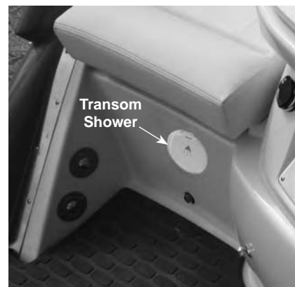
Figure J3: Aft (Transom) Shower
