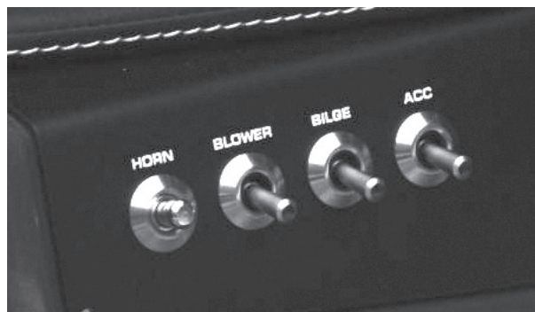
Figure H6: Helm Switch Panel - Port View (Representative View - Models May Vary)
