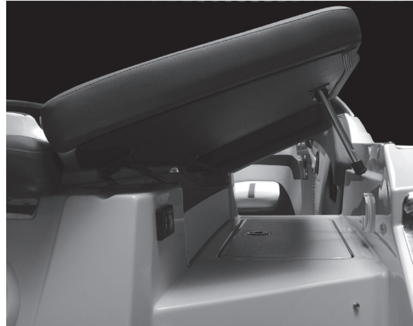
Figure N23: Starboard Sundeck Cushion (Converts to Chaise Lounge - Certain Models Only)
