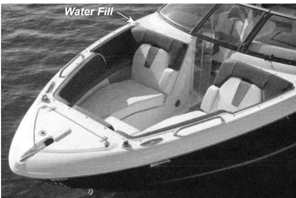
Figure J2: Water Fill - Stbd Windshield Shelf
