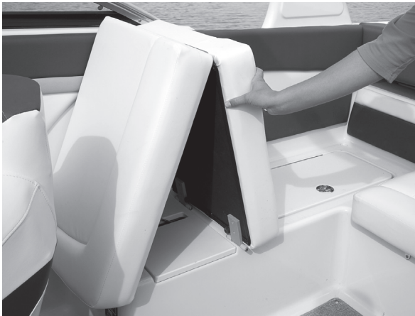
Figure M18: Hinged Seat Cushion - Certain models Only (Creates Step & Provides Access to Storage)
