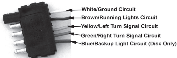
Figure S7: 5-Wire Plug Harness
