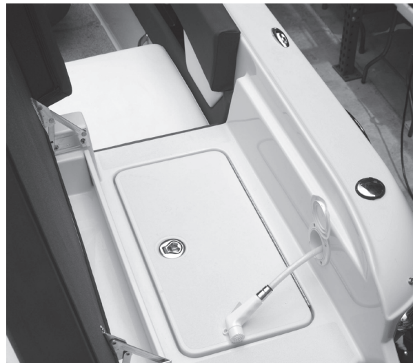
Figure J7: Aft (Transom) Shower
