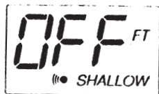
Figure B9: Shallow Alarm
