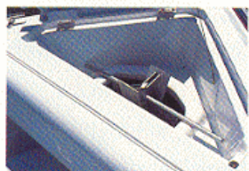
Bow anchor locker with molded anchor well provides quick, easy access and holds anchor securely in place when not in use. New lid is finished both sides and includes a new latch that causes less wear on gelcoat.
