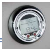
DEPTH SOUNDER WITH AIR AND WATER TEMPERATURE READINGS LETS YOU MONITOR CONDITIONS.
