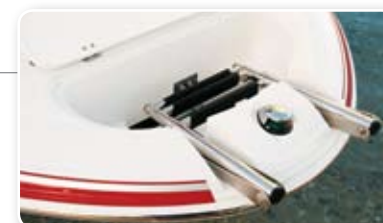
ANCHOR LOCKER/HIDDEN LADDER
