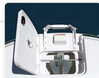
ANCHOR LOCKER/HIDDEN LADDER
