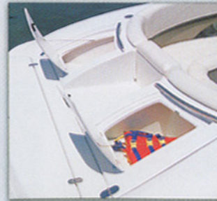
Transom platform lockers
