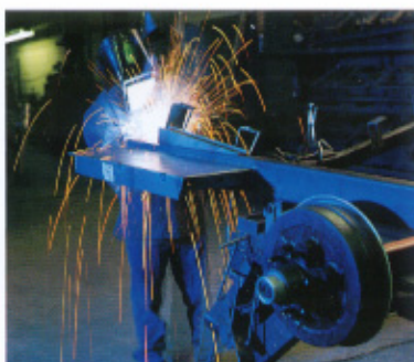
FULLY WELDED TUBE STEEL FRAMES
