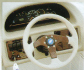
Above: Four Winns exclusive integrated instrument panel with VDO instruments including depth gauge are standard on the 238 and 258 Vista.
