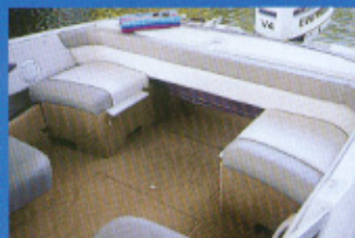
Center section removes, leaving wing seats.
