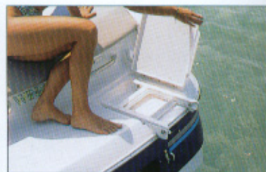
Ladder folds and stores in recessed, hinged compartment.
