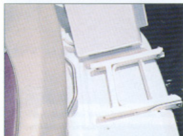
Recessed storage for ladder
