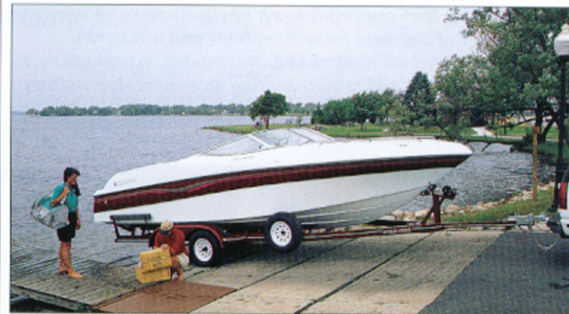
A low profile aids at launch time, often allowing the boat to be floated off the trailer.
