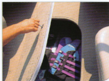
In-floor ski/kneeboard locker
