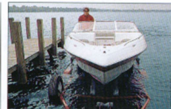
Positioning of side guides, angled bunks and a recessed, frame-mounted roller make it easy to drive the boat onto the trailer.
