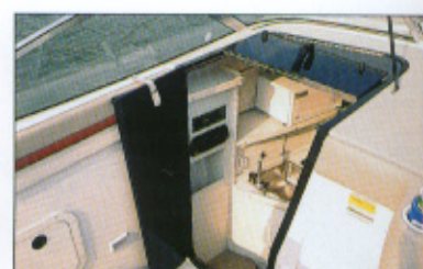
Cabin entry doors open overhead, providing additional light to cabin.
