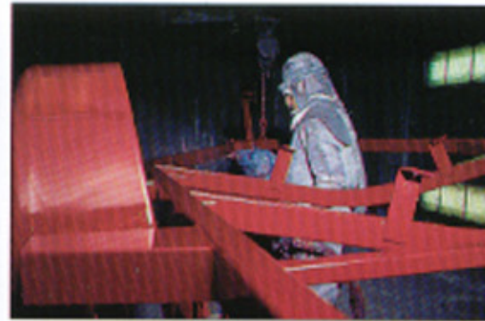
A zinc chromate primer and two coats of color-matched polyurethane paint provide the trailer's outstanding looks and durability.
