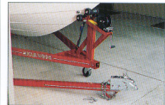
The trailer tongue can be removed, making the trailer length less than the boat's (also provides an added measure of safety and security).
