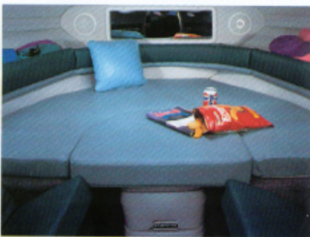
201 cabin has canted seating for extra headroom. Area converts to a berth for two with fill-in cushions. Porti-potti optional.
