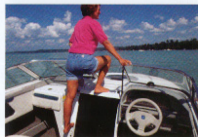
Molded steps in the bulkhead provide access to the deck through a walk-through windshield.
