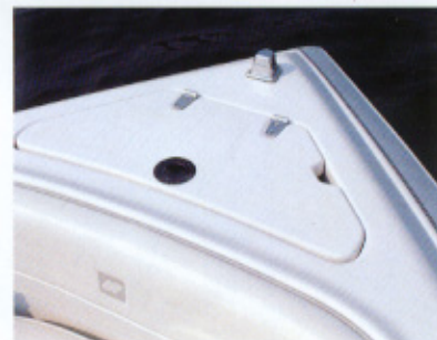
Bow anchor locker has a cradle to isolate the anchor from the fiberglass.
