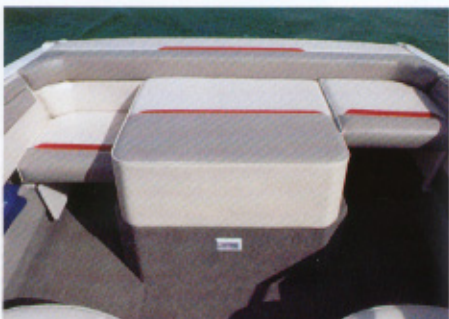
The motor box has a flip-up lid for easy engine access when checking fluid levels, belts and hoses.
