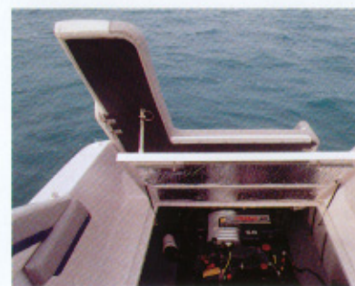
Engine access is convenient through a huge floor hatch.
