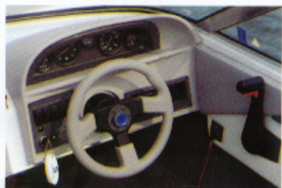
Full instrumentation is fitted in a visored housing for reduced glare.
