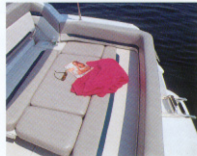
Fill-in cushions combine with the slide out aft-facing seat and stern couch to make a recessed sun lounge.
