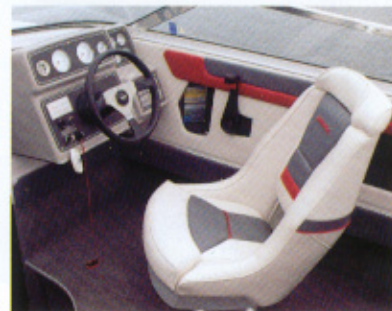
Helm features VDO instrumentation. Highback contoured bucket has side bolsters for lateral support.
