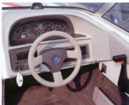
Helm features a new automotive-type dash with shroud for reduced glare and printed circuit instrumentation.
