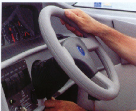
Optional tilt steering wheel is convenient for operators of different physical stature.
