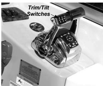
Figure F2: Digital Throttle Shift Control (DTS)
