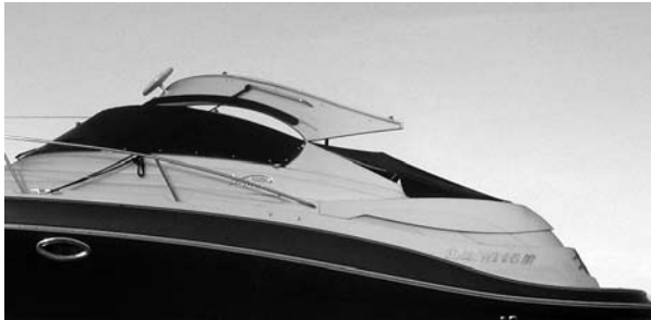
Figure M17: Radar Arch in Resting/Travel Position
