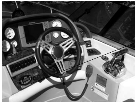
Gasoline Vapors - Blower Warning Label
