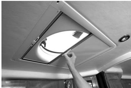
Figure K1: Layered Deck Hatch Screen/Sun/Shade System
