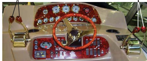
Figure F3: Inboard Helm Station
