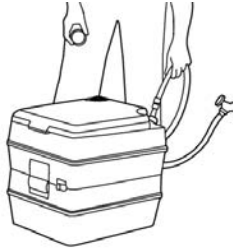
Figure J10: Filling Fresh Water Tank
