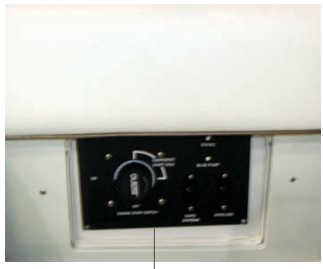
Battery Selector Switch Location (Remove Access Door Stbd Backrest Insert)
