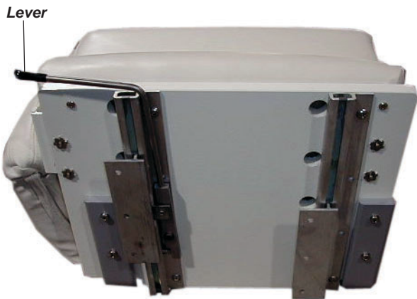
Figure N8: Helm Seat Slider Mechanism
