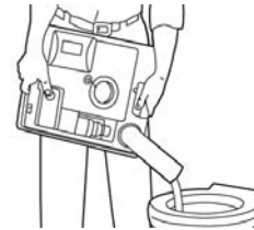
Figure J13: Emptying Waste Holding Tank
