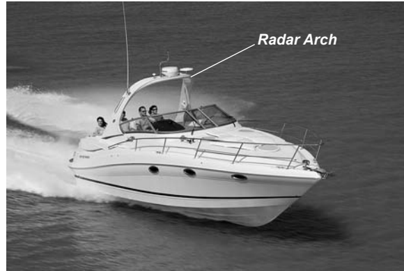
Figure M15: Radar Arch
