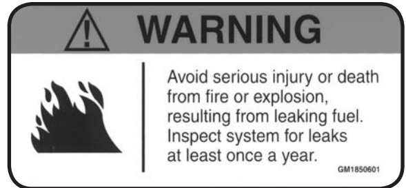
Leaking Fuel Warning Label
