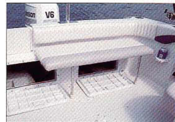
Transom access to battery and oil reservoir
