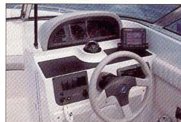
Automotive-style instrumentation with planned area for optional fish finder and electronic add-ons
