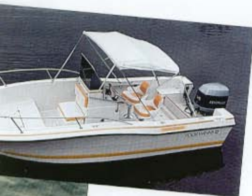
Standard canvas top provides protection from the sun. (shown: CC w/Bimini top)
