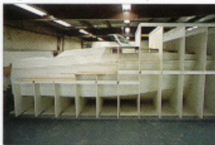
Full scale modeling helps us define interior content before models are built
