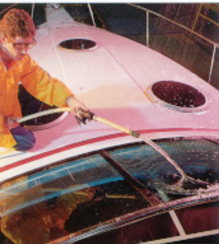
"Storm" testing the 315 Vista for leaks
