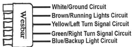
Figure P7: 5-Wire Plug Harness
